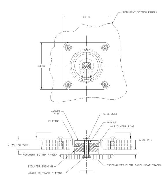
JMCS-010-010-001 INSTALL KIT, SEAT TRACK, ISOLATED .75 PANEL THICKNESS JMCS-010-010-031 INSTALL KIT, SEAT TRACK, ISOLATED .50 PANEL THICKNESS
