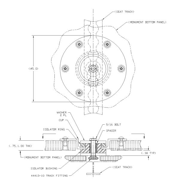
JMCS-010-012-001 INSTALL KIT, SEAT TRACK MOUNT, ISOLATED .75 PANEL THICKNESS JMCS-010-012-003 INSTALL KIT, SEAT TRACK MOUNT, ISOLATED .50 PANEL THICKNESS
