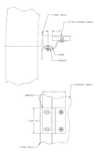
JMCS-010-010-067 INSTALL KIT, 3" DIM "A" JMCS-010-010-035 INSTALL KIT, 6" DIM ""A"
