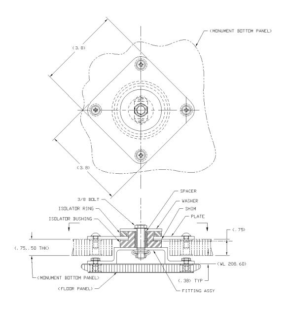
JMCS-010-010-003 INSTALL KIT, FLOOR PANEL, ISOLATED .75 PANEL THICKNESS JMCS-010-010-033 INSTALL KIT, FLOOR PANEL, ISOLATED .50 PANEL THICKNESS
